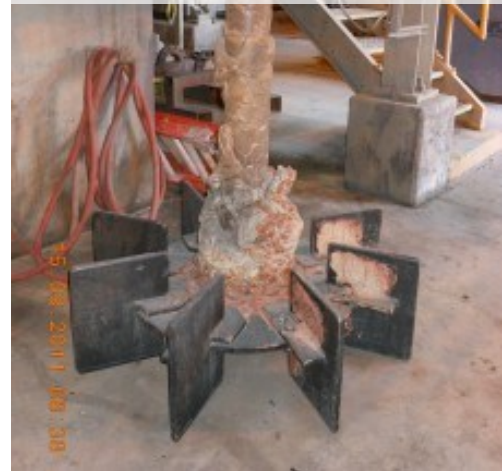
Watson Coated Titanium Autoclave Agitator Blades & Disc—50 months runtime
