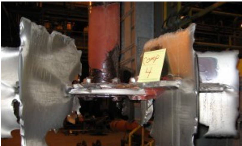
Un-coated 3/4 Titanium Autoclave Agitator Blades & Disc—9 months run time (84RPM gearbox)
